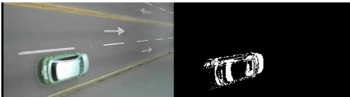
Figure 5 Example input and output of background subtraction
